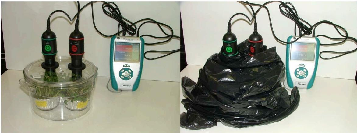
Fig. 2. Illustrating measurement of CO<sub>2</sub> and O<sub>2</sub> (optional) concentrations in both light and dark conditions. These measurements were taken in a 2000-mL biochamber available from Vernier Instruments, but could be taken in any reasonably airtight container large enough to hold a number of photosynthesizing plants.
